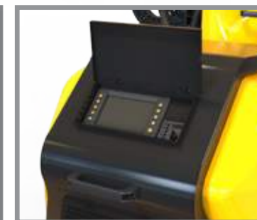
The control panel features a large display used for advanced hydrodemolition settings and the engine ignition and throttle
