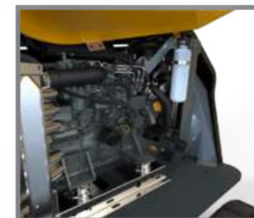
The engine service area is completely accessible by opening the left side hatch
