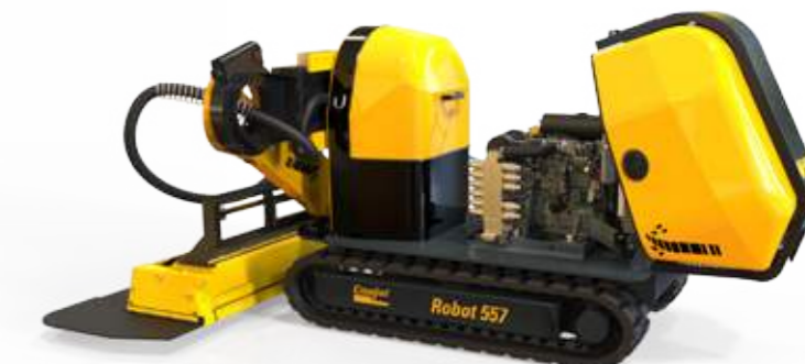
For thorough maintenance and repair, the whole hood can be tipped backwards
